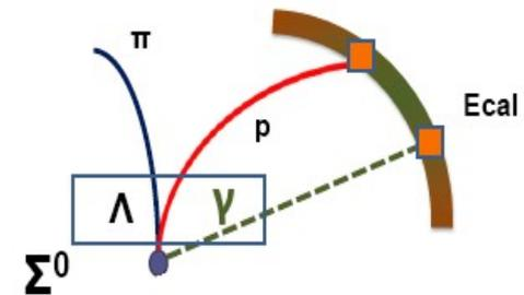
2) only events occurring in the gas filling the chamber are selected by cutting on the  $\Lambda$  decay vertex position ( $r_\Lambda > 30$  cm) taking into account for the maximum path of the  $\Lambda$  and the error on the vertex position.
