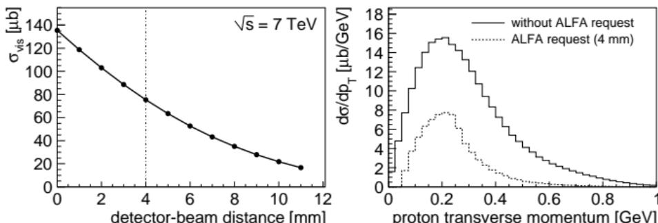
Left: Cross section visible in the ALFA detectors (both protons tagged) as a function of the distance between the detectors and the beam centre. Distance of 4mm corresponds to 75  $\mu\text{b}$  of cross-section visible in the ALFA detectors.
