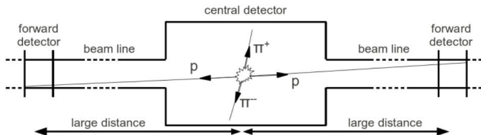
Pions detected in the ATLAS detector (tracker or calorimeter).
