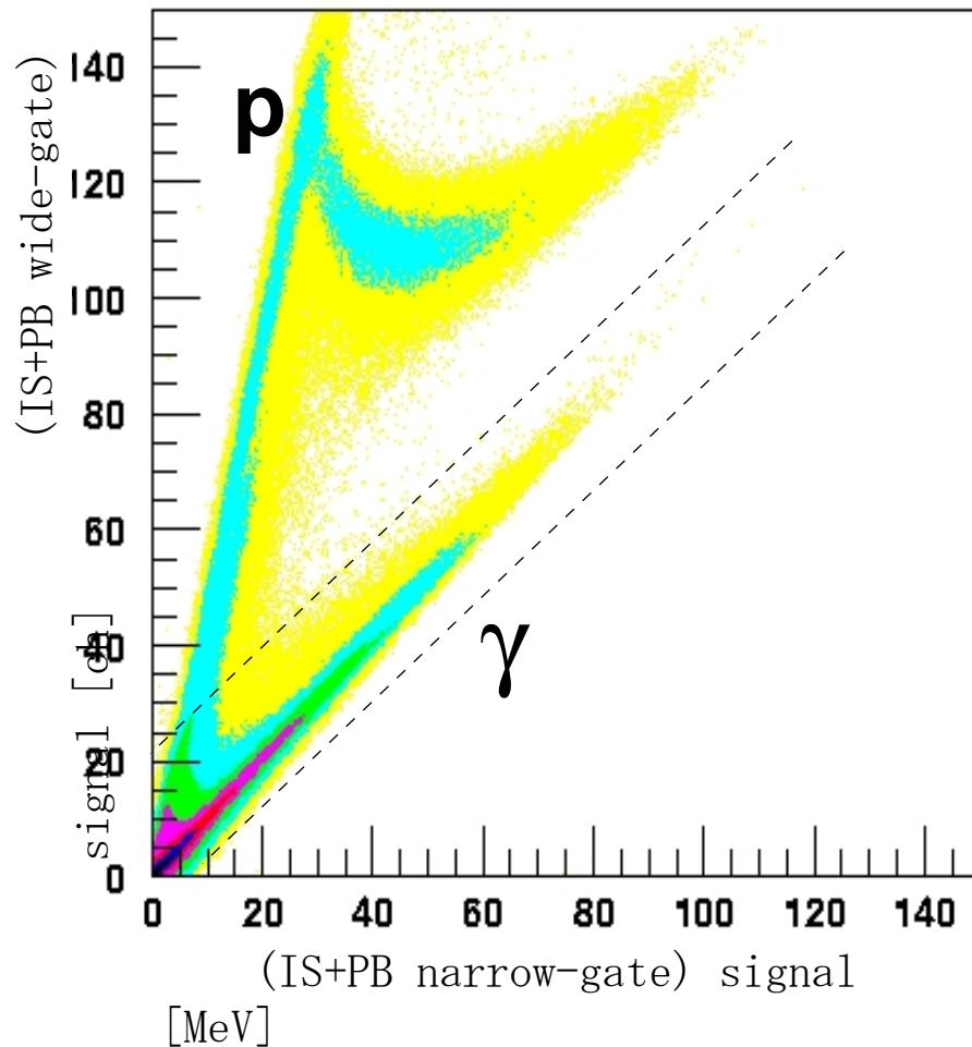
Photon identification from the Plastic Ball pulse shape
