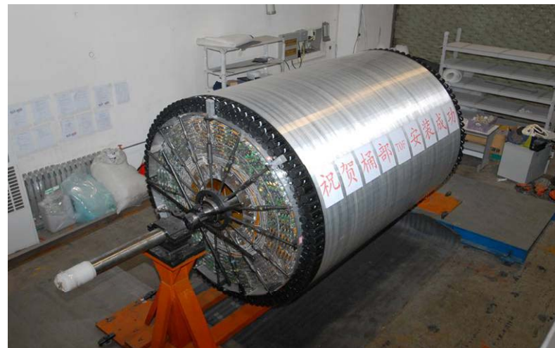
Structure of Barrel TOF
