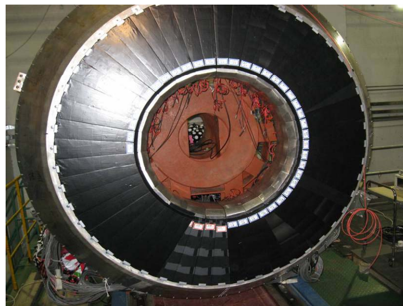
Structure of Endcap TOF
